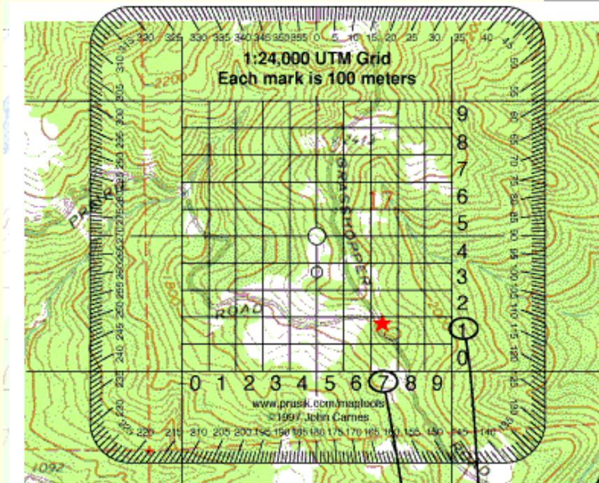
This is a grid overlay tool laid on top of a map. It is made for the 24000:1 scale maps and is see through plastic. The small blocks divide the 1000 meter square we worked with before into 100 meter square blocks leaving us to estimate only within the 100 meter square box giving much more accuracy. You see the Red Star covers about 30 by 30 meters so we don't even try to get it to 1M accuracy.
