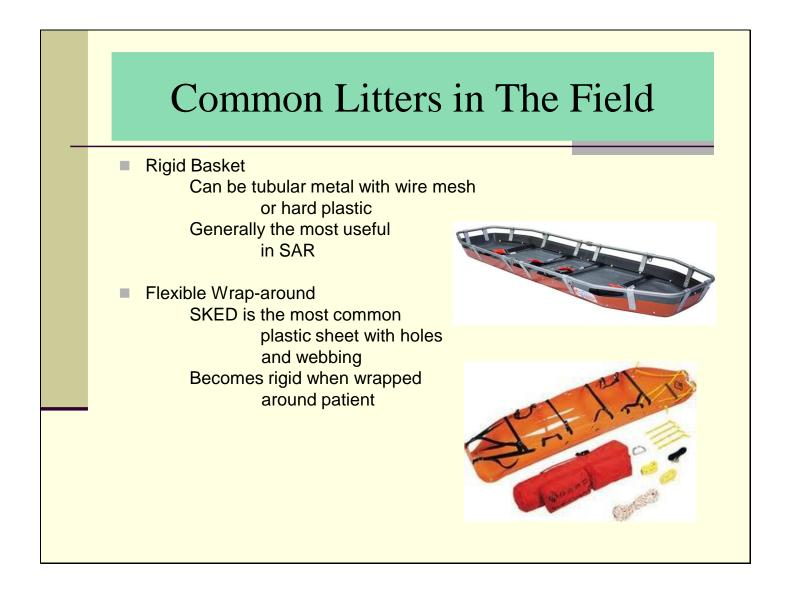
Generally, rigid basket stretchers will all have a metal frame. Some have wire mesh forming the basket, others have plastic composites or fiberglass.
