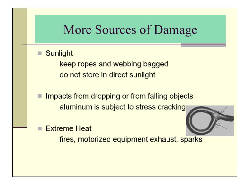
Rope is also degraded by prolonged exposure to sunlight.
